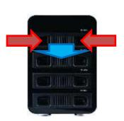
1. Pull out the tray module and install the hard drives
