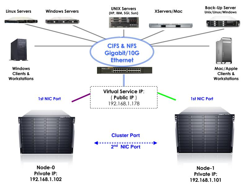
It is <u>Real Time</u>, <u>Synchronized</u>, <u>Block level</u>, <u>Volume base</u> data replication with automatic <u>Fail-Over</u> from one node to another node. It can be viewed as if a RAID-1 across 2 NAS units over LAN.
