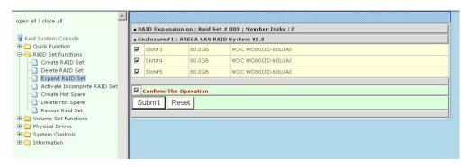
To expand a raid set, click on the **Expand Raid Set** link. Select the target raid set, which you want to expand it.
