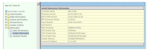
Use this feature to view the raid subsystem controller's information. The controller name, firmware version, serial number, main processor, CPU data/Instruction cache size and system memory size/speed appear in this screen.
