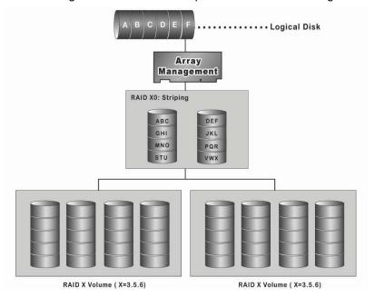
RAID level-X0 allows more physical drives in an array. The benefits of doing so
