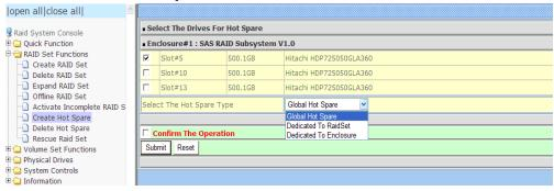
When you choose the **Create Hot Spare** option in the Raid Set Function, all unused physical devices connected to the current controller appear: Select the target disk by clicking on the appropriate check box. And Select the Hot Spare type as Global, Dedicated Raid or Dedicated Enclosure. Tick on the **Confirm The Operation**, and click on the **Submit** button in the screen to create the hot spares.
