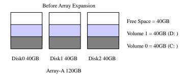
The RAID subsystem controller redistributes the original volume set over the original and newly added disks, using the same fault-tolerance configuration. The unused capacity on the expanded raid set can then be used to create an additional volume set, with a different fault tolerance setting if user needs to change.
