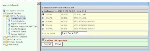
To create a raid set, click on the **Create Raid Set** link. A **Select The SAS (SATA) Drive For RAID Set** screen will display showing the drives connected to the current controller. Click on the selected physical drives with the current raid set. Enter 1 to 15 alphanumeric characters to define a unique identifier for a raid set. The default raid set name will always appear as Raid Set. #.
