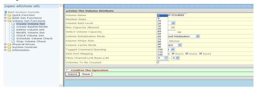
**Fibre LUN:** Each Fibre LUN base can support up to 8 LUNs. Most Fibre Channel host adapter treats each LUN like a Fibre disk.
