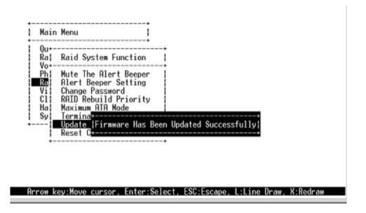
10. After the new firmware completes download, user should find a chance to restart the controller for the new firmware to take effect.
