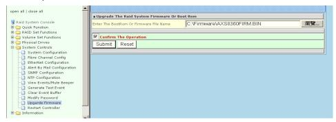
After the firmware upgrade is complete, a bar indicator will show "Firmware Has Been Updated Successfully"
