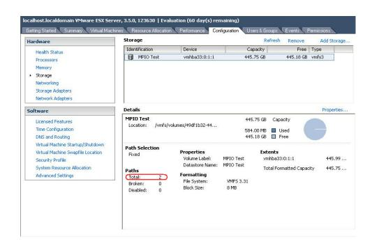
Step 13: Click "Properties...." of "vmhba33:0:1:1" to manage MPIO. In this case, Vmhba33:0:1 is the first path; vmhba33:1:1 is the second path
