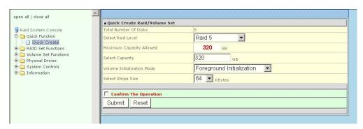
The number of physical drives in the raid subsystem determines the RAID levels that can be implemented with the raid set. You can create a raid set associated with exactly one volume set. The user can change the raid level, stripe size, and capacity. A hot spare option is also created depending upon the existing configuration.
