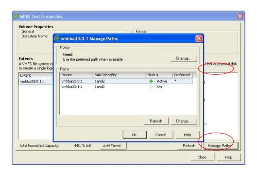
Step 15: Preferred path "Enabled" or "Disabled." When MPIO Policy "Fix" is chosen, one path will be auto assigned as the preferred path (Active), and the other path will be automatically assigned as "Standby." "Fix" is the default MPIO Policy.
