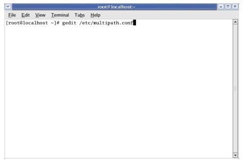
Modify the vendor name and product name. In this example, the vendor name should be "Sans Digital" and the product name should be "AR316F8R-VOL#\*". Save it then reboot the host server computer. If the Sans Digital AccuRAID SAS-to-SAS redundant controller RAID subsystem is tested here, in this example, the vendor should be as "Sans Digital" and the product name should be "AR316X6R-VOL#\*".
