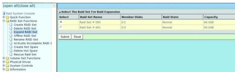
2. Select the target RAID set by clicking on the appropriate check box. Select the target disk by clicking on the appropriate check box.
