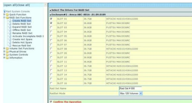
128 volumes is the default mode for SAS RAID controller, the 16 volumes mode is used for support roaming this raidset to SATA RAID controllers. The SATA RAID controller is designed to support up to 16 volumes only. You have to use “Max 16 volumes” on the raidset mode if you plan to roam this raidset between SAS RAID controller and SATA RAID controller.
