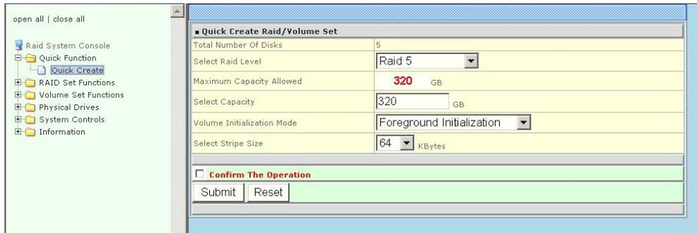
The number of physical drives in the raid subsystem determines the RAID levels that can be implemented with the raid set. You can create a raid set associated with exactly one volume set. The user can change the raid level, stripe size, and capacity. A hot spare option is also created depending upon the existing configuration.
