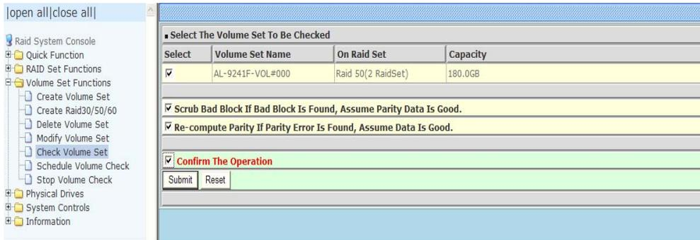
**Scrub Bad Block If Bad Block Is Found, Assume Parity Data Is Good** option: the check button will be shown when Data disk found bad blocks, and if selected, the RAID controller will regenerate data from Parity disk to data disk, if check button not yet selected RAID controller will report error only.
