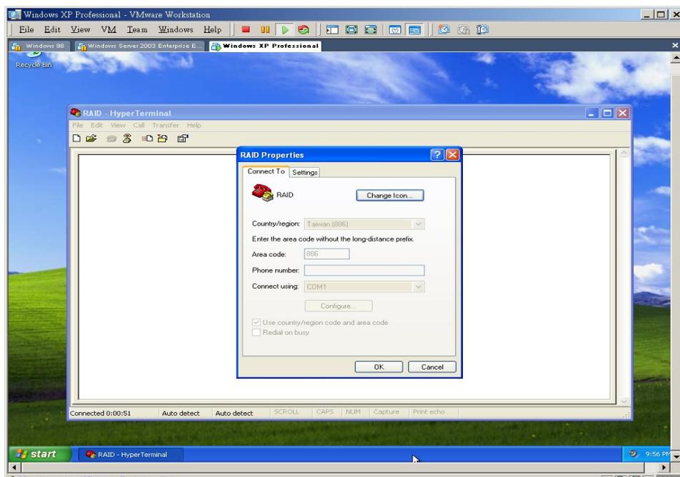
Step 8. Open the Settings Tab. Function, arrow and ctrl keys act as: Terminal Keys, Backspace key sends: Ctrl+H, Emulation: VT100, Telnet terminal: VT100,
