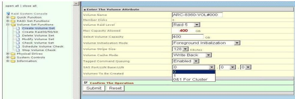
**SAS LUN base:** Each SAS wide port device is attached to the SAS card. A SAS wide Port can connect up to 128(0 to 127) devices. The RAID subsystem is as a large SAS device. We should assign a LUN base from a list of SAS LUNs.
