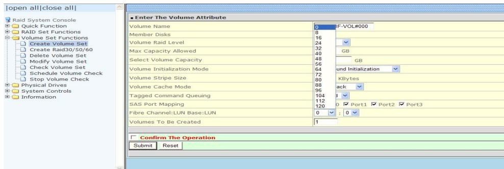
**Fibre LUN:** Each Fibre LUN base can support up to 8 LUNs. Most Fibre Channel host adapter treats each LUN like a Fibre disk.
