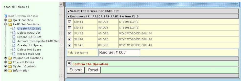
To create a raid set, click on the **Create Raid Set** link. A **Select The SAS (SATA) Drive For RAID Set** screen will display showing the drives connected to the current controller. Click on the selected physical drives with the current raid set. Enter 1 to 15 alphanumeric characters to define a unique identifier for a raid set. The default raid set name will always appear as Raid Set. #.
