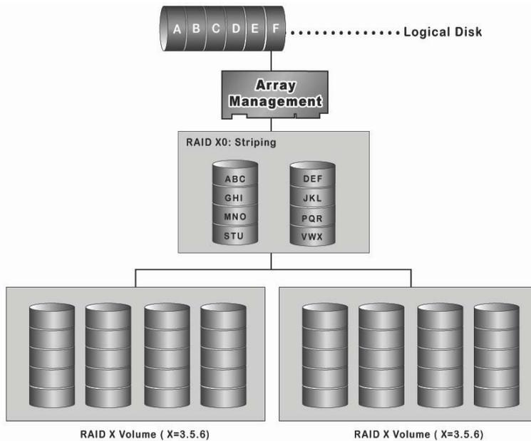
RAID level-X0 allows more physical drives in an array. The benefits of doing so
