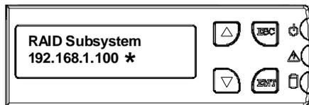
After push “Down arrow button” three times then you can read the message of LCM from 2<sup>nd</sup> Controller :
