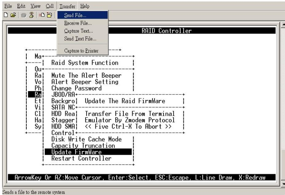
4. Select “**ZMODEM modem**” under Protocol. ZMODEM as the file transfer protocol of your terminal emulation software.
