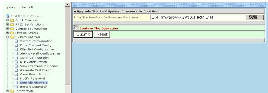
After the firmware upgrade is complete, a bar indicator will show “Firmware Has Been Updated Successfully”
