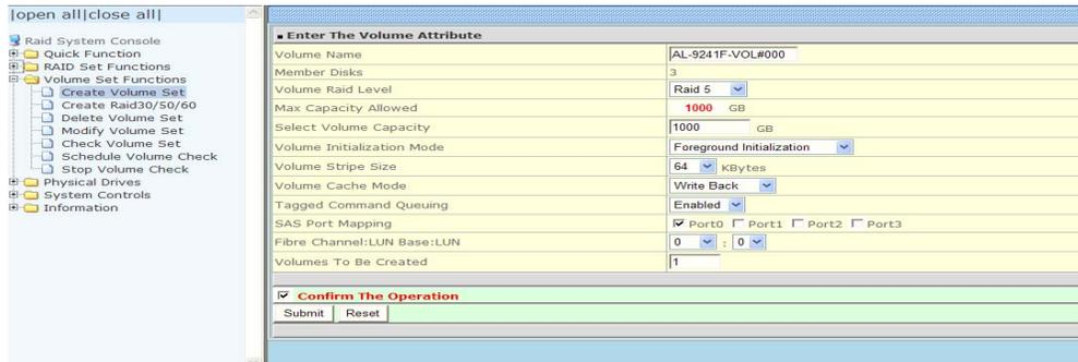
**Fibre LUN base:** Each Fibre device attached to the Fibre card, as well as the card itself, must be assigned a unique Fibre ID number. A Fibre channel can connect up to 128(0 to 127) devices. The RAID subsystem is as a large Fibre device. We should assign a LUN base from a list of Fibre LUNs.
