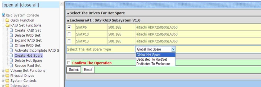
When you choose the **Create Hot Spare** option in the Raid Set Function, all unused physical devices connected to the current controller appear: Select the target disk by clicking on the appropriate check box. And Select the Hot Spare type as Global, Dedicated Raid or Dedicated Enclosure. Tick on the **Confirm The Operation**, and click on the **Submit** button in the screen to create the hot spares.
