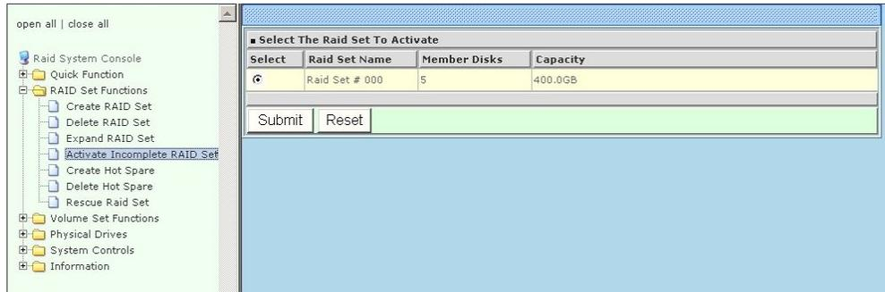
Click on the **Submit** button in the screen to activate the raid set that has removed one of the disk drives in the power off state. The RAID subsystem will continue to work in degraded mode.
