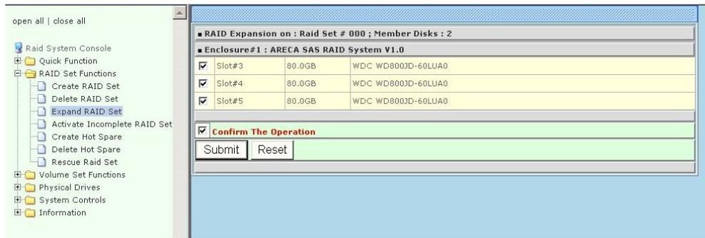
To expand a raid set, click on the **Expand Raid Set** link. Select the target raid set, which you want to expand it.
