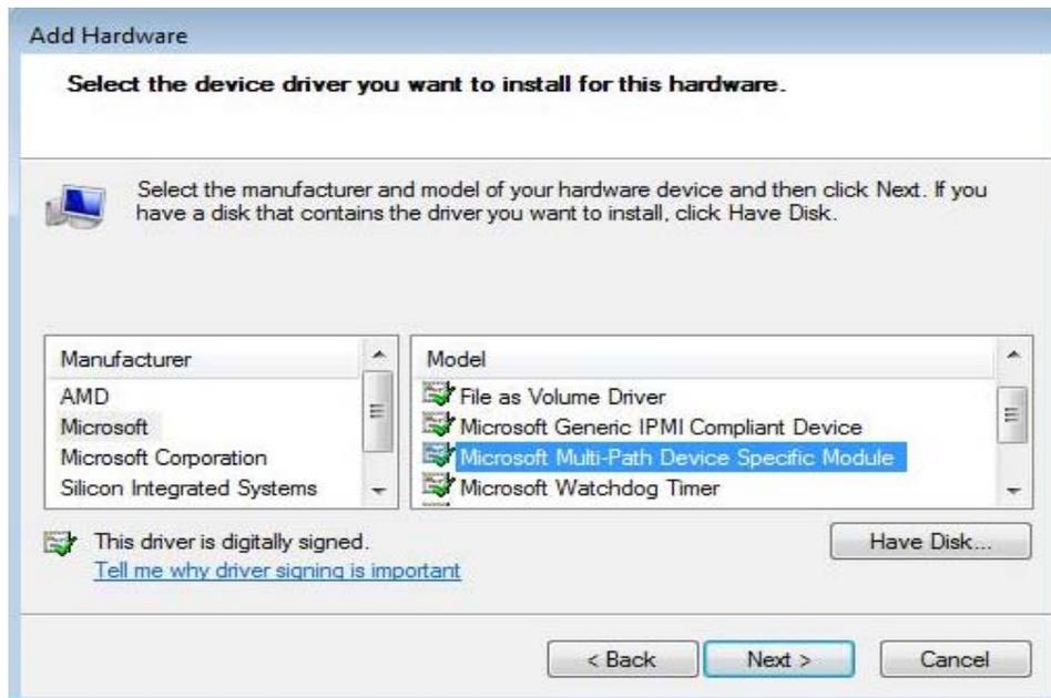
Follow the wizard to complete installing “Microsoft Multi-Path Device Specific Module”.
