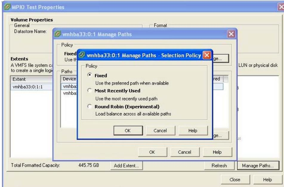
Step 17: Now, the data storage with dual path failover support setting is done; the users could start installing new virtual machine into this data storage.
