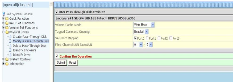
After you complete the selection, tick on the **Confirm The Operation** and click on the **Submit** button to complete the selection action.
