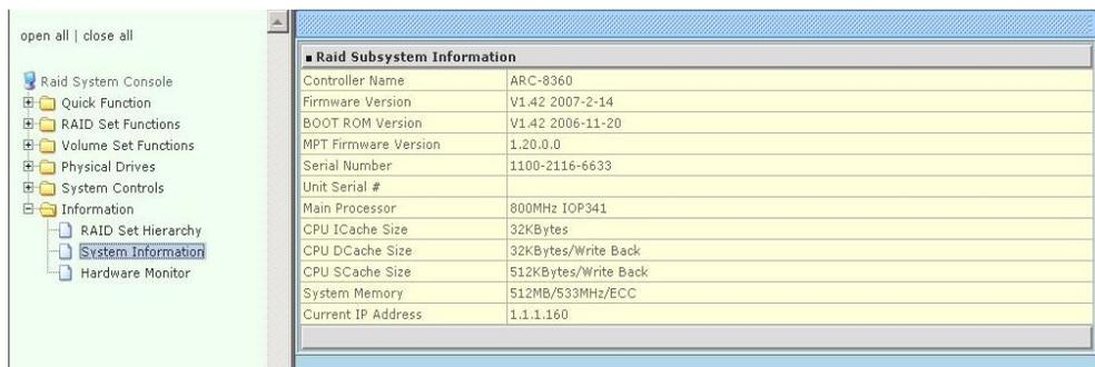
Use this feature to view the raid subsystem controller’s information. The controller name, firmware version, serial number, main processor, CPU data/Instruction cache size and system memory size/speed appear in this screen.
