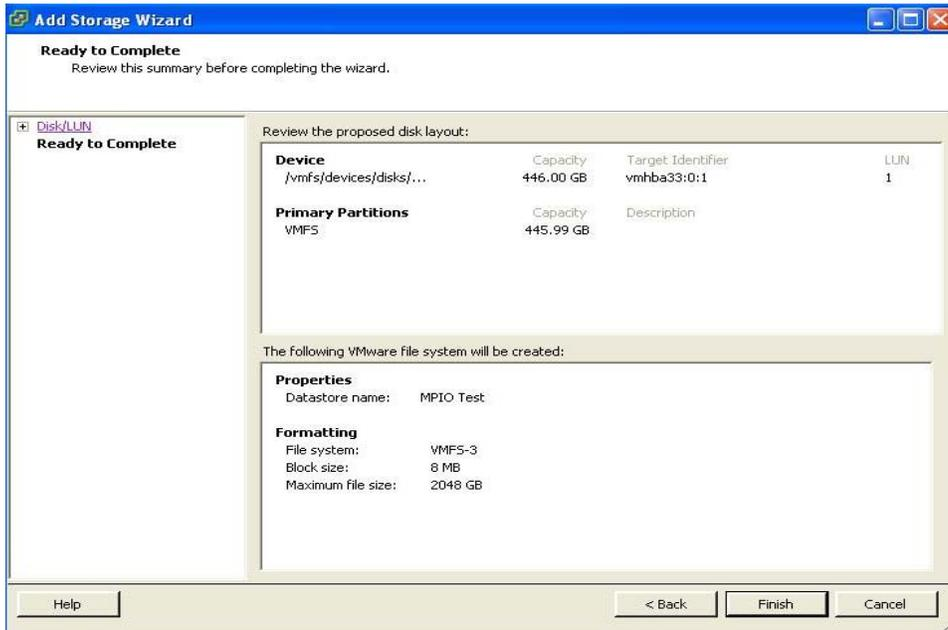
Step 12: Now the storage device “vmhba33:0:1:1” is able to be used, and it has two I/O paths. If only one path available, that means either “0&1 For Cluster” is not pre-set on the RAID subsystem or one of the dual host ports on the Fibre HBA or the RAID controller is linked down
