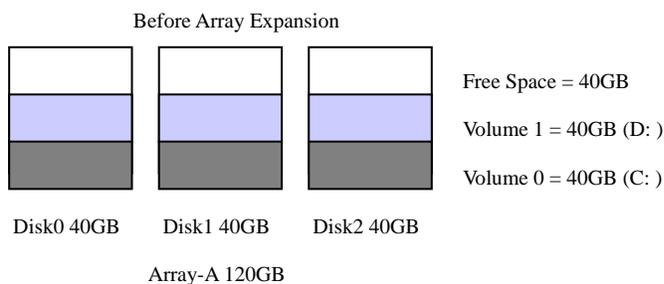
The RAID subsystem controller redistributes the original volume set over the original and newly added disks, using the same fault-tolerance configuration. The unused capacity on the expanded raid set can then be used to create an additional volume set, with a different fault tolerance setting if user needs to change.
